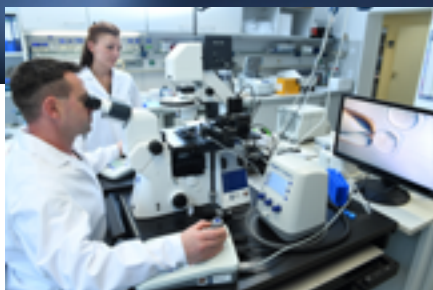
Team members perform microinjections on mouse embryos using micromanipulators equipped with micropipettes.
