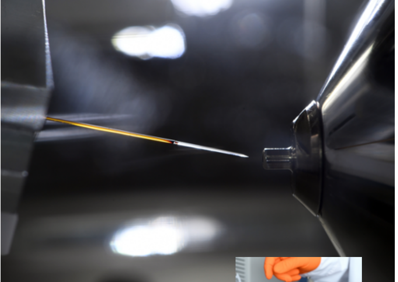
This precision device, which couples liquid chromatography and mass spectrometry, is used to identify and quantify proteins.
